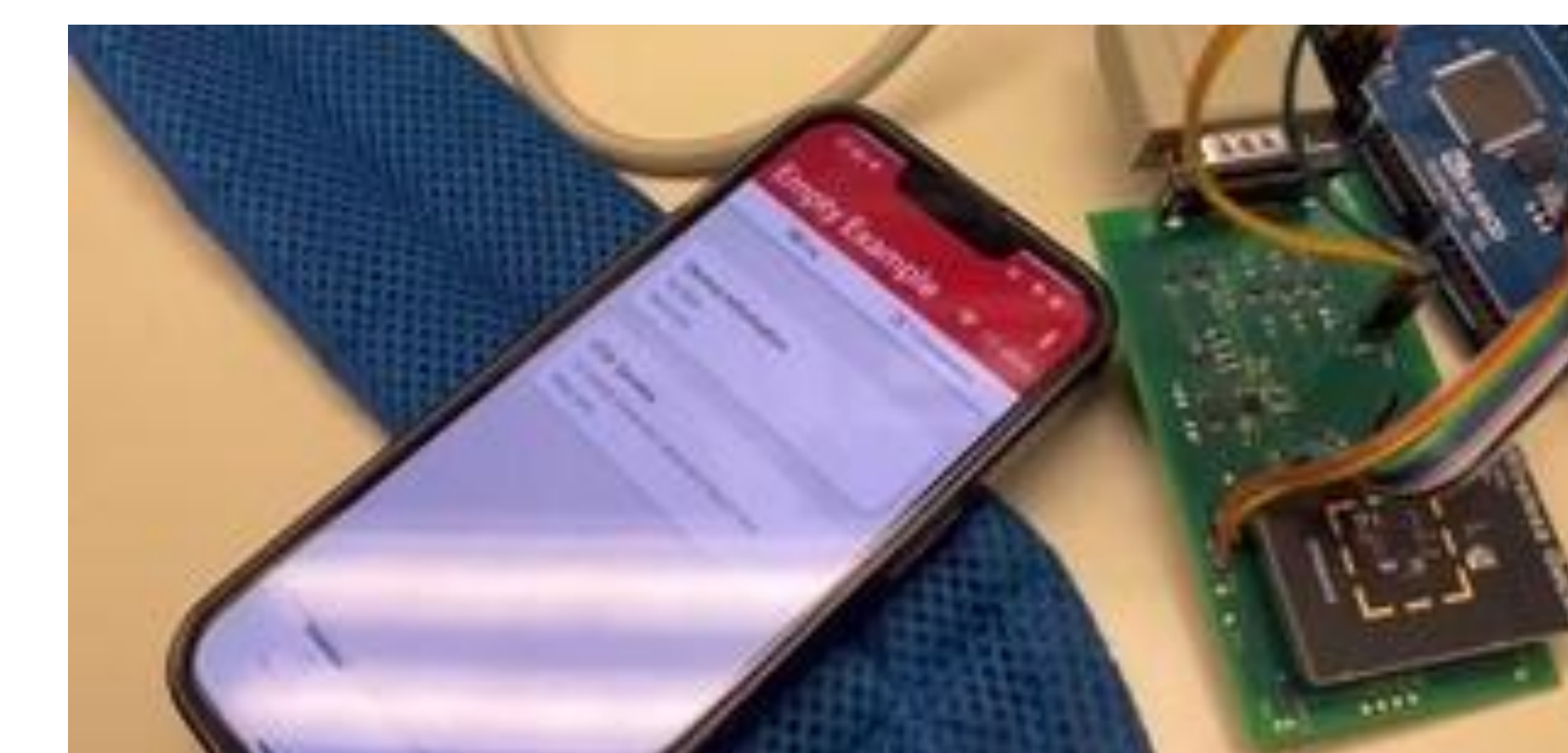
Fig. 6 Building stable Bluetooth connection with cellphone and our device
